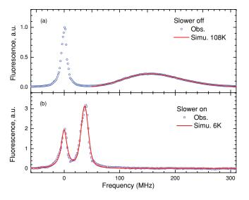
FIG. 3. (Color online) LIF signal observed 230 cm downstream in the MOT chamber. The slower beam was off for (a) and on for (b).
